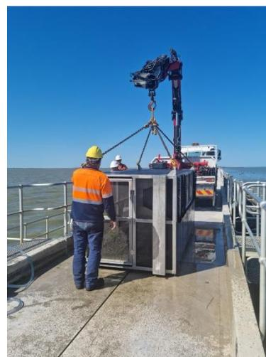
Figure 4: Cage trap used to sample lamprey migrating through the barrage fishways (DEW)
